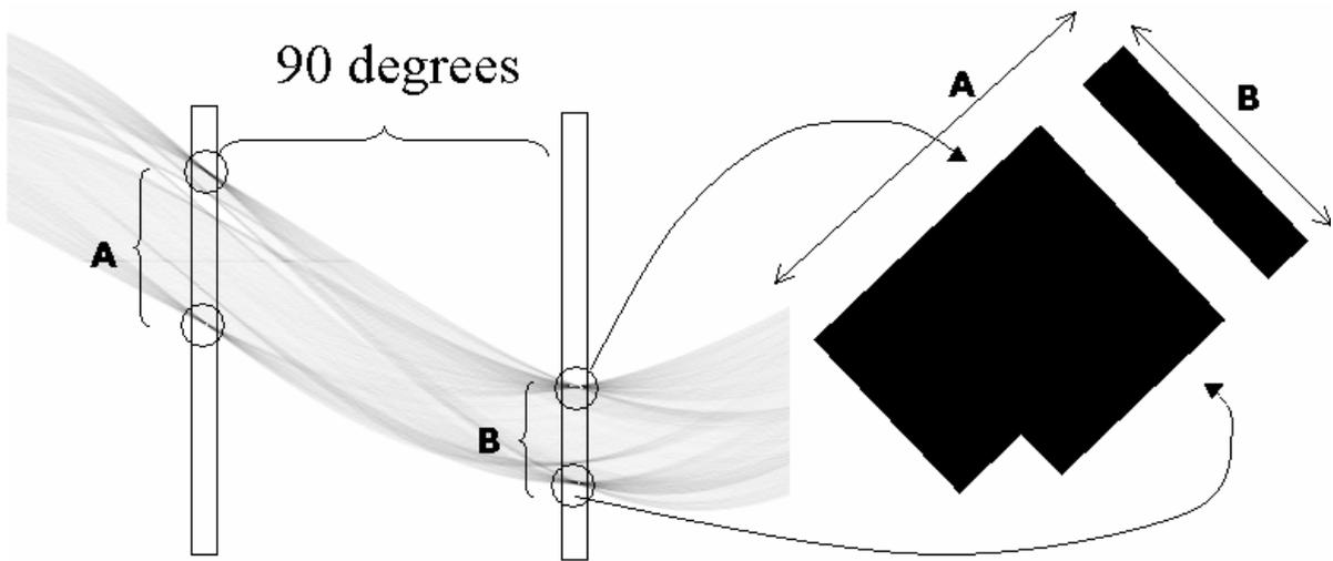
Figure 6: Representation of the Hough transform of a segmented box. In this image the relation between the desired measures and the maxima of the accumulation space can be easily seen.
