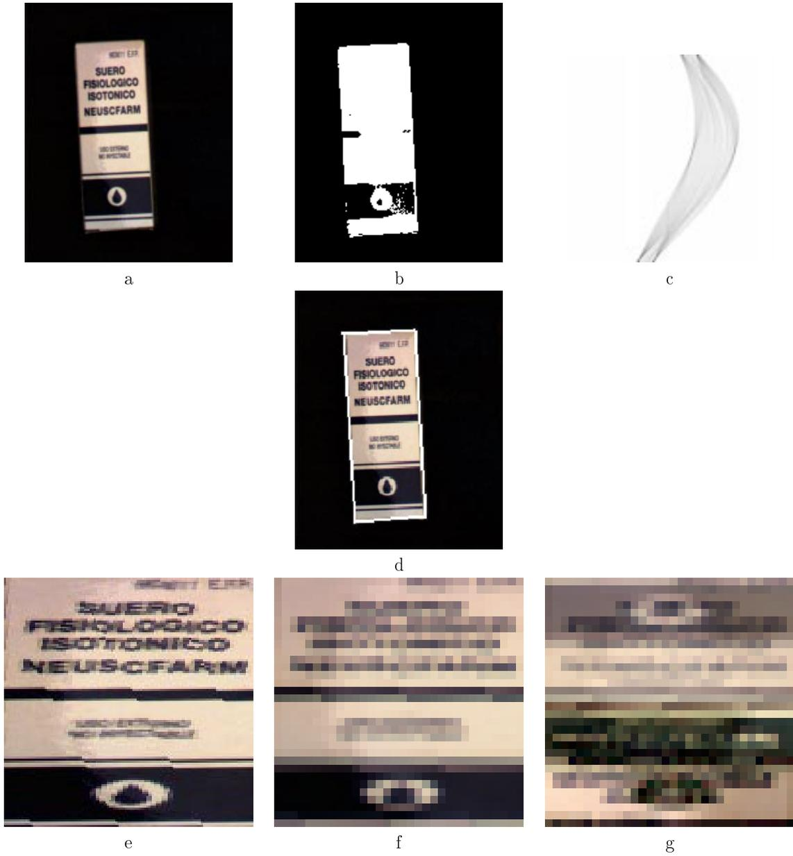
Figure 5: Object segmentation. (a) Original image, (b) Segmented blobs, (c) Hough transform of blob edges, (d) Detected rectangle, (e) Normalized image, (f) Sampled ( $32 \times 32$ ) normalized image, (g) Invariant image representation.
