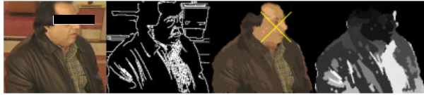
Fig. 2. Original image, contour image, quantization, initial regions.
