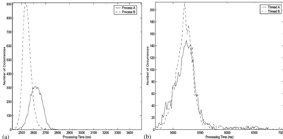
Fig. 9. Distribution of the execution time of (a) 2 processes and (b) 2 threads, using a dual processor PIII-600 MHz.
