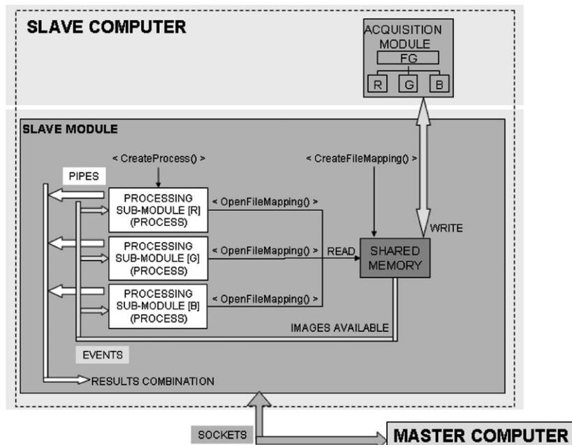
Fig. 3. Communication involved in the PC-based modular architecture.
