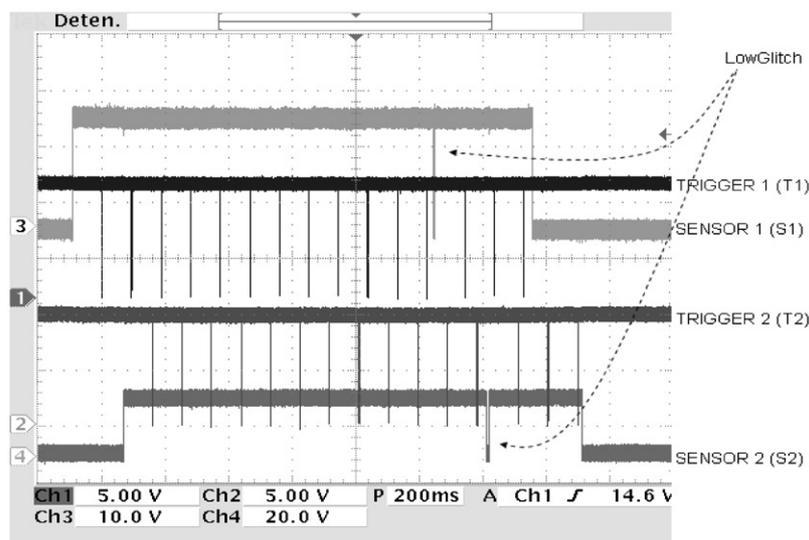
Fig. 8. Result of digital filtering.
