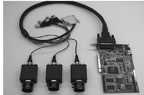
Fig. 2. Modular acquisition system.
