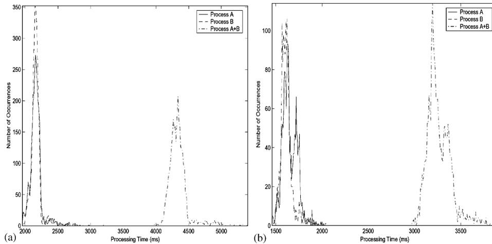
Fig. 10. Distribution of the execution time of two sequential processes using (a) a single processor PIII-800 MHz and (b) a single processor PIV-1.8 GHz.
