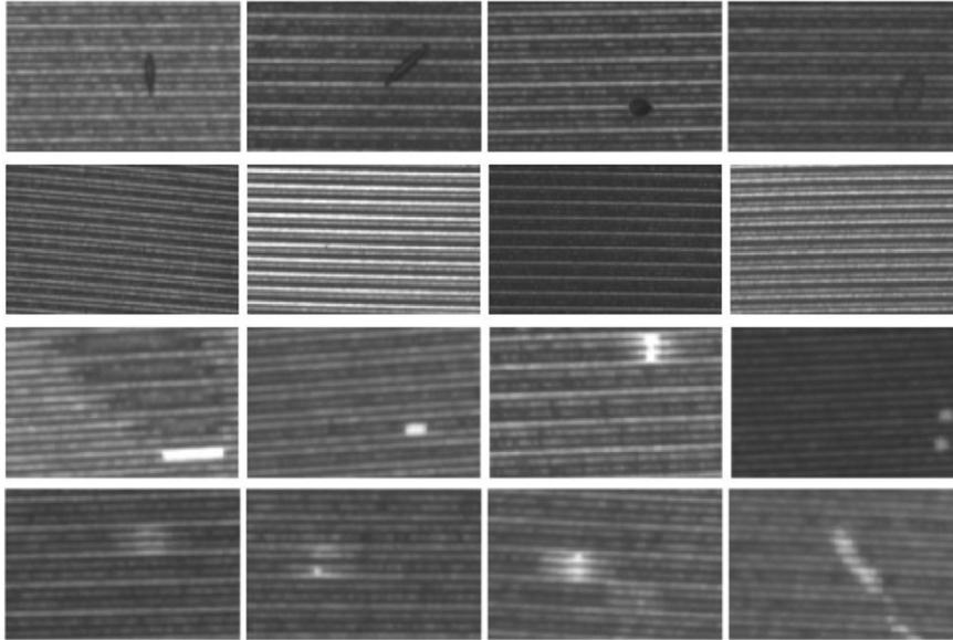
Fig. 4. Some examples of defects to be detected: (a) bubbles, (b) landing, (c) line-out and (d) line reduction, respectively.
