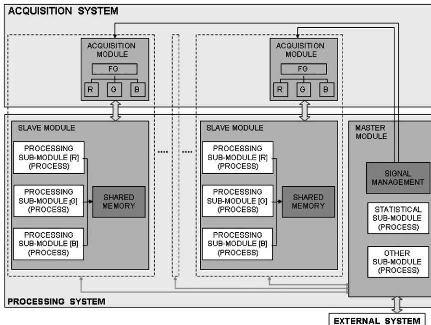
Fig. 1. Modular architecture of a PC-based vision system.
