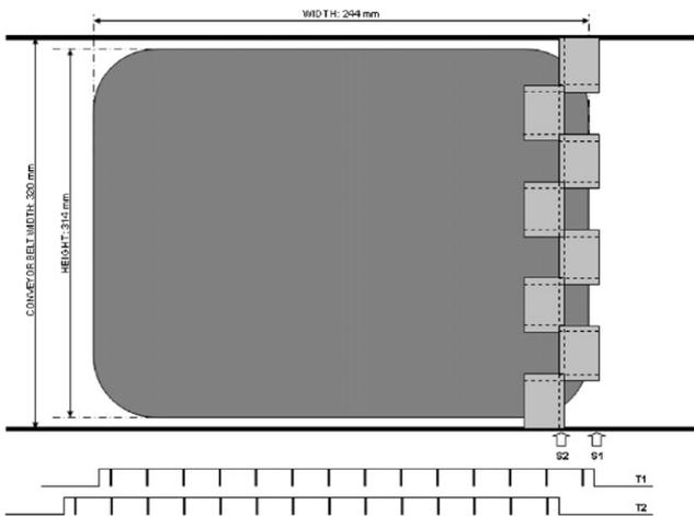
Fig. 6. Acquisition configuration: two lines of four cameras triggered by signals T1 and T2 that depend on the sensor signals S1 and S2, respectively.
