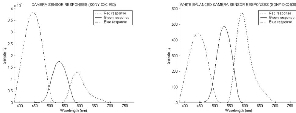
FIG. 1. Sensitivities of the SONY DXC-930 camera used to generate the RGB values of the colour samples selected to build the learning set. Left: Original sensitivities of the camera. Right: White balanced camera responses.
