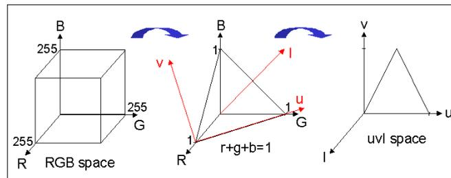
FIG. 2. Scheme of the transformation from the RGB colour space to the  $uvI$  space.
