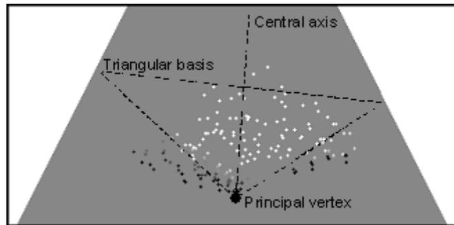
FIG. 4. Chromatic categories have a triangular basis with a principal vertex and a central axis. In the central area of the triangular basis, samples have membership values near one. In the areas near the two sides of the triangle that share the principal vertex membership values decrease from one to zero.
