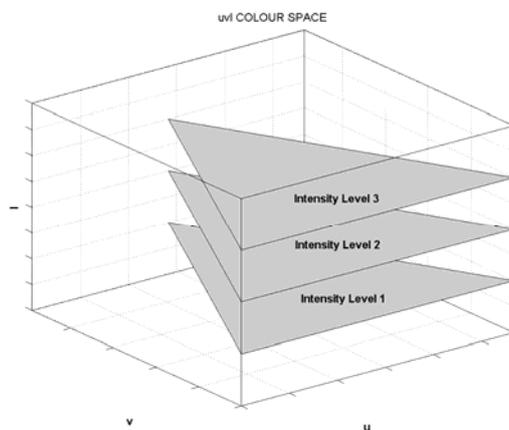
FIG. 7. Scheme of the division of the  $uvI$  colour space in three levels of intensity. All the samples inside a level of intensity are represented and modelled with the sigmoid-gaussian function on a 2D  $uv$ -plane.
