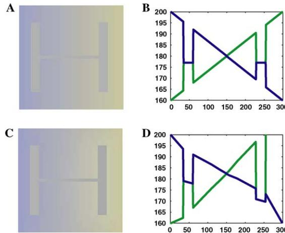
Fig. 10. (A) Original image, (C) perceptual sharpening of (A). (B,D) present a profile of an horizontal line of images (A,C), respectively.
