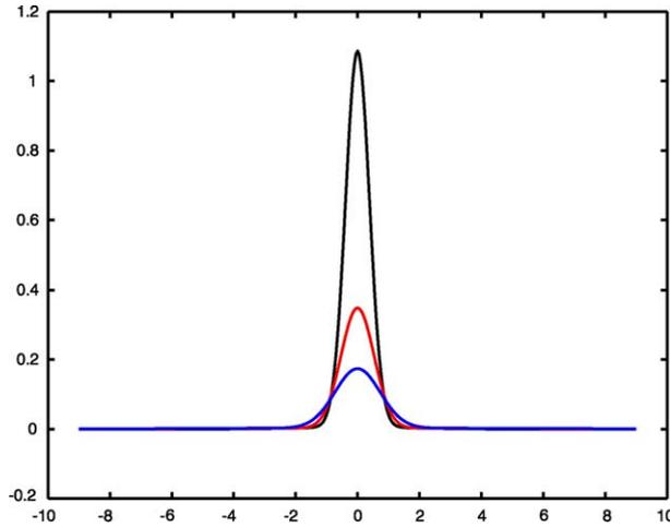
Fig. 7. Example of profiles of the 2D symmetric filters for the Spatial-CIELAB. Black, red, and blue colour lines represent the kernel for the intensity, red-green, and yellow-blue channel, respectively. (For interpretation of the references to colour in this figure legend, the reader is referred to the web version of this paper.)
