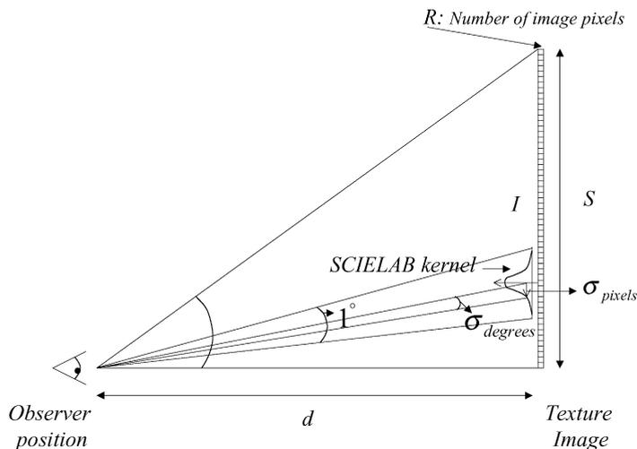
Fig. 6. General scheme for unit conversion from visual angle to image pixels.
