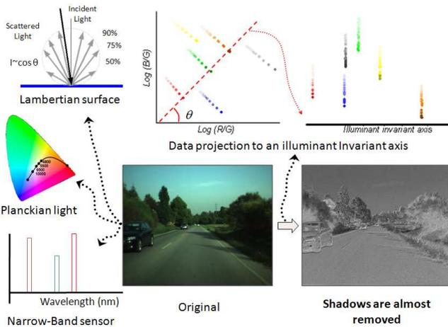
Fig. 2. Under the assumptions of Planckian light, Lambertian surface and narrow-band sensors, we can obtain an illuminant-invariant image which is almost shadow free.
