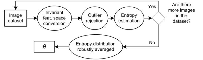
Fig. 6. Algorithm to calibrate the camera using road images. Given a group of images, the entropy distribution is calculated as the robust mean over different entropy distributions. The invariant angle ( $\theta$ ) is the minimum of the final robustly-averaged entropy distribution.
