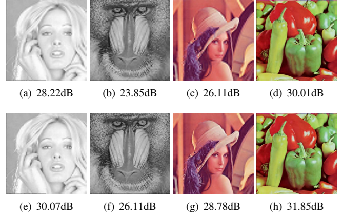
Fig. 6. Examples of reconstructed images compressed by means of JPEG2000 (a-d) and Hi-SET (e-h) at 0.17bpp (a & e), 0.86bpp (b & f), 0.39bpp (c & g) and 1.05bpp (d & h).
